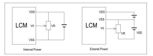
$V_{DD-}V_0$ : LCD Driving voltage VR: 10k~20k
